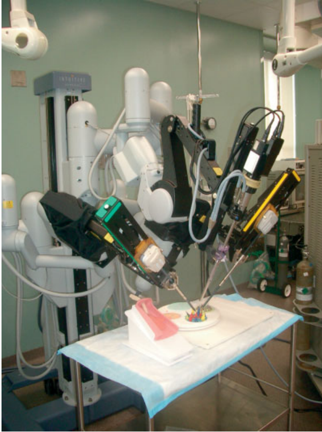
Figure 1. Da Vinci® surgical system in preparation for practice session. [Color figure can be viewed in the online issue, which is available at www.interscience.wiley.com .]
